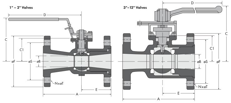
NOTE: Gear Operators are suggested on size 10" and 12" valves.  $\textbf{NOTE:} \ A \ trunnion-like \ Ball \ Support \ is \ included \ on \ size \ 12'' \ valves.$
